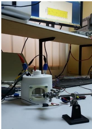
Figure 1. Photoelectrochemical cell with three electrodes
